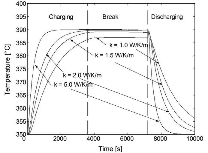
Fig. 5: Influence of thermal conductivity of storage material on storage temperature at distance  $d_a/2$  from tube
