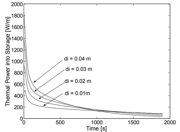
Fig. 10: Thermal power transferred to storage system for various diameters of flow channel
