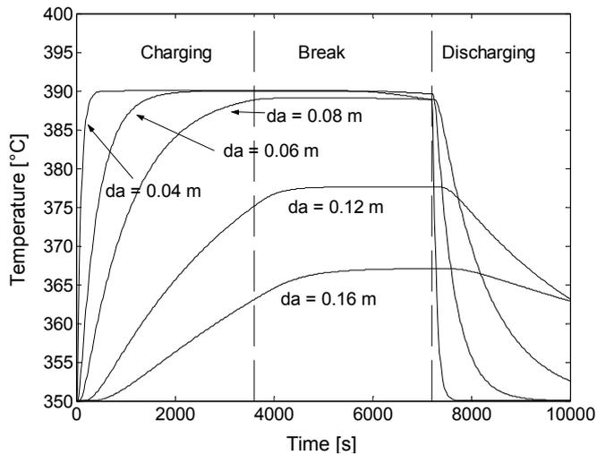
Fig. 11: Influence of distance between flow channels on storage temperature at distance  $da/2$  from tube
