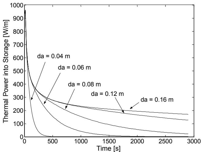
Fig. 12: Thermal power transferred during charging period to storage material for different values for distance between flow channels
