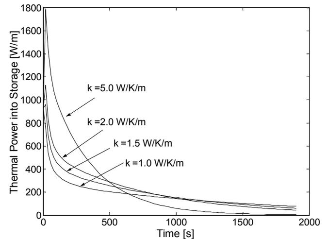
Fig. 6: Thermal Power transferred to differential storage element during charging with varying thermal conductivity of storage material
