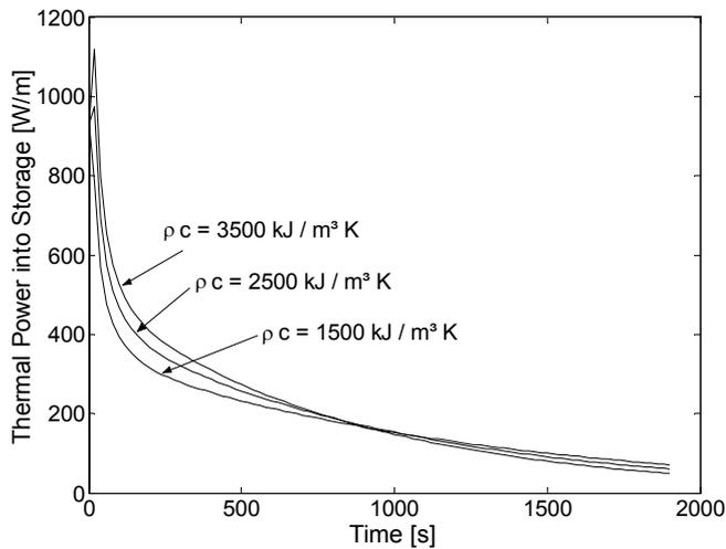
Fig. 8: Influence of volumetric heat capacity on thermal power transferred to storage medium during charging period
