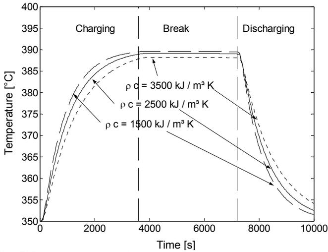
Fig. 7: Influence of volumetric heat capacity on storage temperature at distance  $da/2$  from tube
