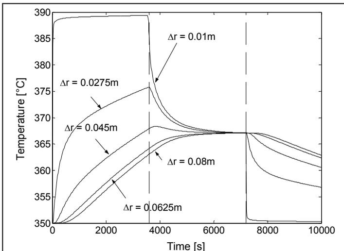
Fig. 13: Temperature in storage material at different distances  $\Delta r$  from flow channel. Distance between axis of flow channels is 0.16 m
