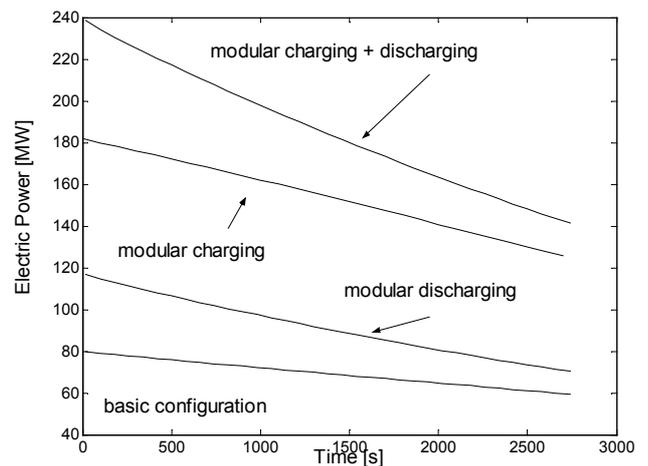
Fig. 20: Calculated values for electric power provided by power plant during discharge for different charging and discharging strategies; identical storage geometry
