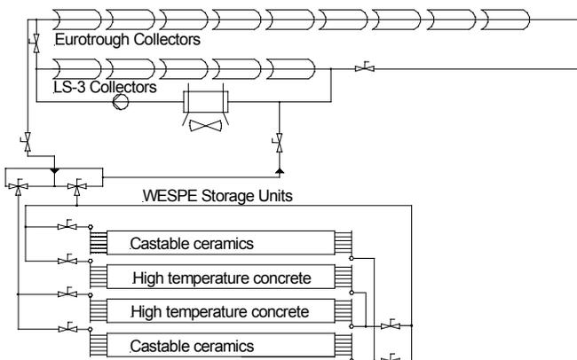
Fig. 2: Integration of test storage units into parabolic trough test loop at PSA
