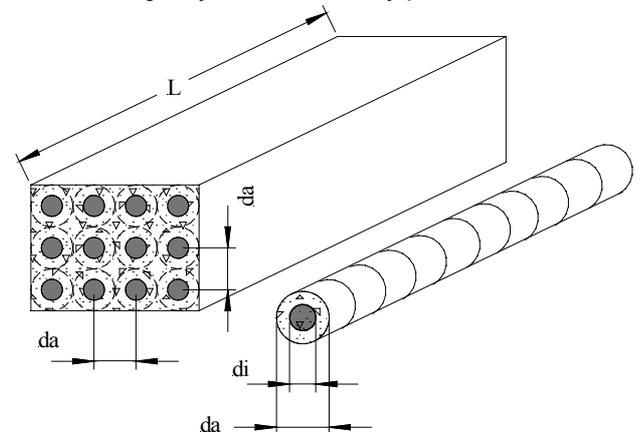
Fig. 3: Physical Model for the storage unit and parameters describing the geometry
