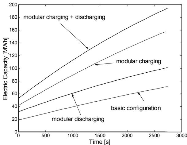
Fig. 21: Results for electric energy provided by power plant during discharge of storage for different charging and discharging strategies; identical storage geometry
