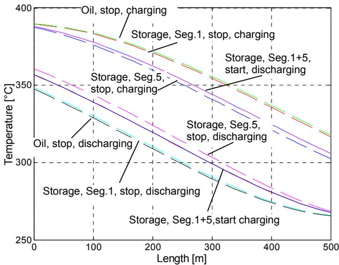
Fig. 14: Temperature distribution in the storage versus length for beginning and end of charging and discharging, respectively
