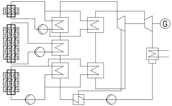
Fig. 19: Modular discharge concept; re-heating at two different temperature levels
