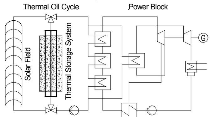
Fig. 1: Basic concept for integration of thermal energy storage into solar thermal parabolic trough power plants
