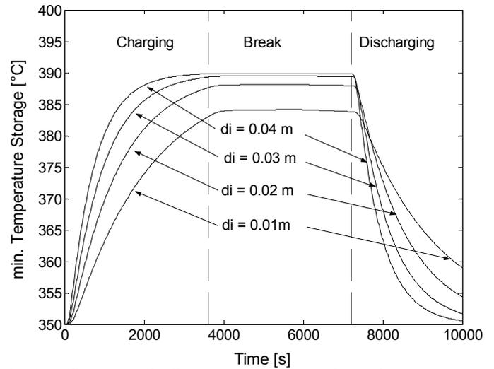
Fig. 9: Influence of diameter of flow channel on storage temperature at distance  $da/2$  from tube
