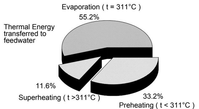
Fig.17: Distribution of thermal energy transferred to feed water of Rankine cycle of parabolic trough power plant
