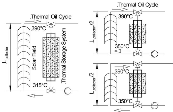
Fig. 18: Configuration solar field: basic concept (left) and modular charging concept (right); exemplary values to show effect on allowable storage outlet temperature
