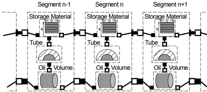
Fig. 4: Part of the Modelica-model representing a single tube and the surrounding storage material. The tube and the storage material are discretized in axial direction, the storage material is also discretized in radial direction
