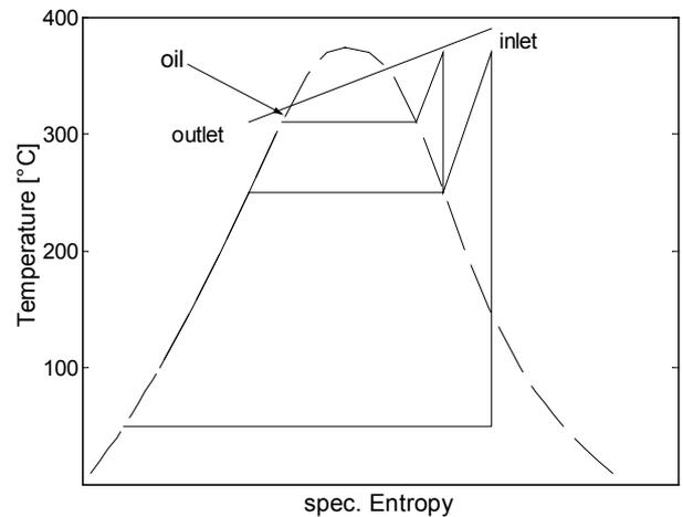
Fig. 16: Power cycle for basic concept in T-s diagram during discharge
